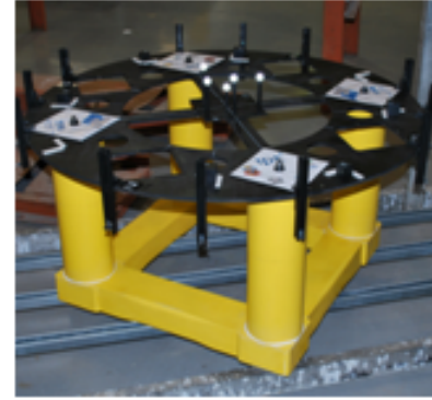
FIGURE 2. Circular column model scale hull used in the model tests and calculations.
